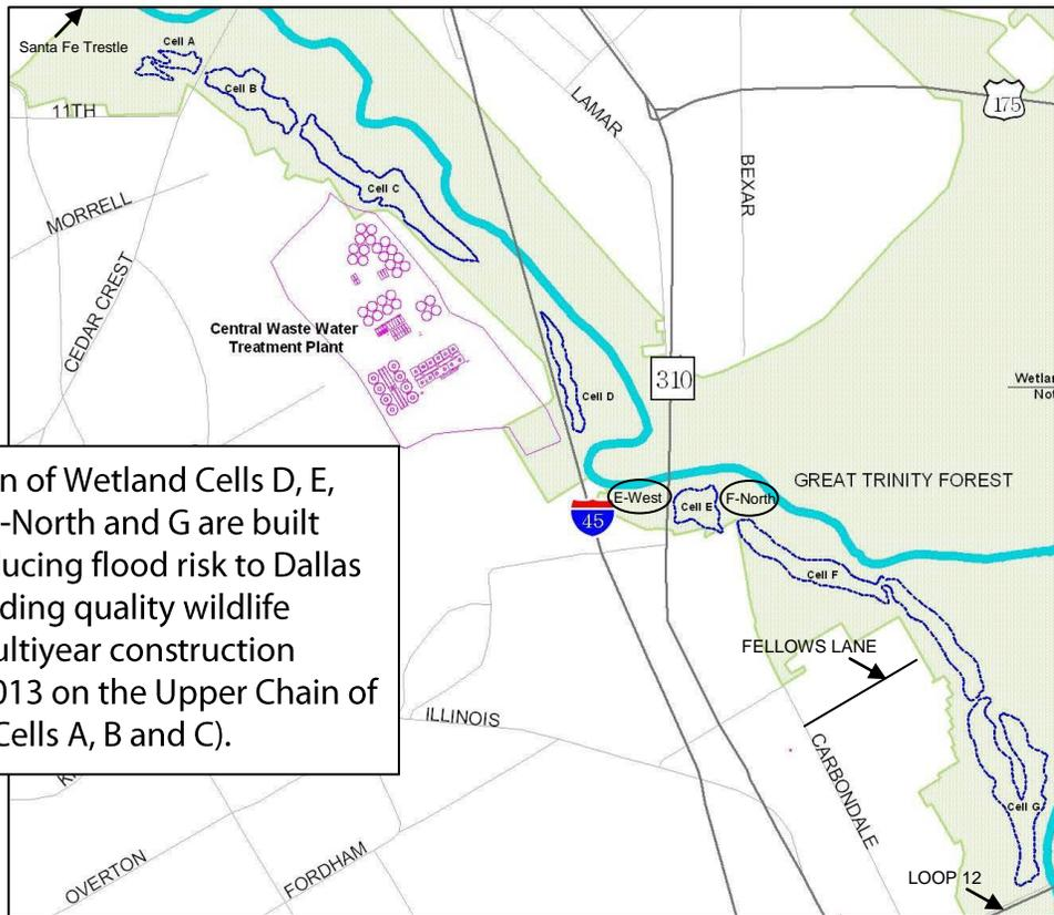
Lower Chain of Wetland Cells D, E, E-West, F, F-North and G are built and are reducing flood risk to Dallas while providing quality wildlife habitat. Multiyear construction began in 2013 on the Upper Chain of Wetlands (Cells A, B and C).
